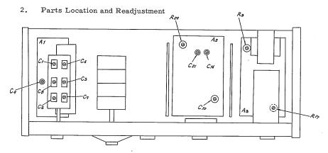
The circuit of this instrument is divided into three printed-circuit boards. The adjusting trimmer capacitors and semi-fixed resistors are located as shown above.
