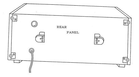
Dismantle the feet by removing the four mount screws on the rear panel. Then it becomes possible to pull out backward the top, bottom, and side plates respectively.
